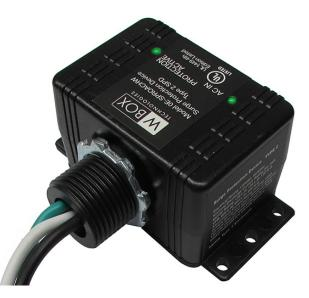
The high performance OE-SPROACHW is a Type 2 Surge Protection Device that protects sensitive electronic loads connected to service panels, intrusion alarm panels, fire panels and devices connected directly to it, via parallel installation on 120VAC branch circuits. LED indicators for AC input and active surge protection. NEMA Type 1 sealed ABS weather and impact resistant plastic enclosure. Lead wires 15". UL1449, 4th Edition listed.
